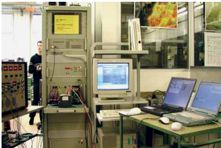
Measurement of the behaviour of the devices in voltage dips, brief interruptions or voltage fluctuations of the power supply
